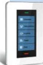
UbiQ-231 comes with a 4.3" flat touch panel design scenario control panel, Built-in IR receiver, RS-485, LAN and USB ports for versatile connectivity, and more optional functions. It runs Windows CE or Linux.
