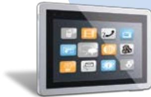
UbiQ-481 comes with a 11.6" flat touch panel design scenario control panel, with rich I/O (USB, dual LAN, RS-232/485, Video-in and Line-in/out), an IR receiver, echo cancellation, and more optional function. It runs Windows CE or Linux.
